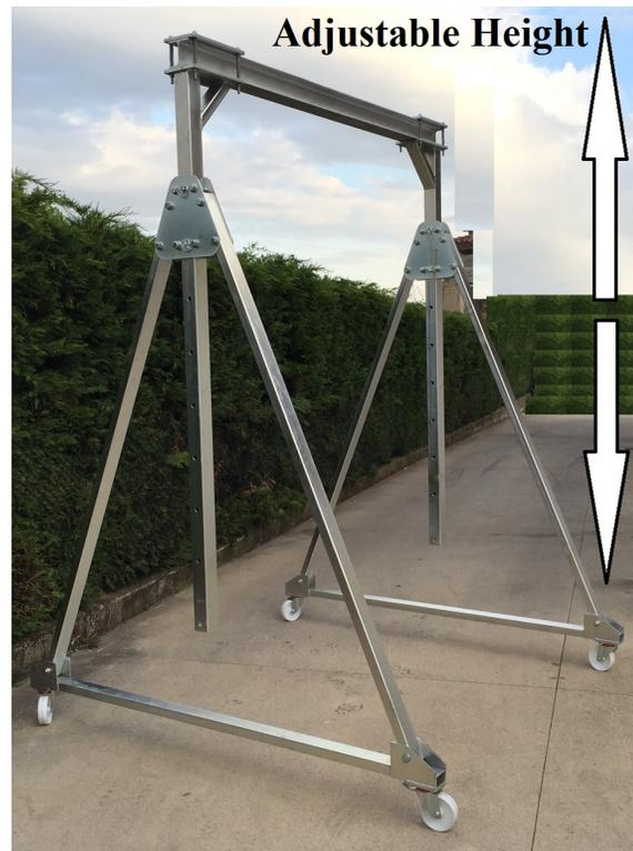
Gantry cranes are equipped with electro-industrial wheels swivel on double ball, with hub on a double ball and rolling band reported vulcolan to ensure maximum smoothness of industrial floor smooth; the wheels are equipped with integrated holding brake to bring the crane up to 2000 kg while for higher capacities are supplied 2 wheel chocks.
